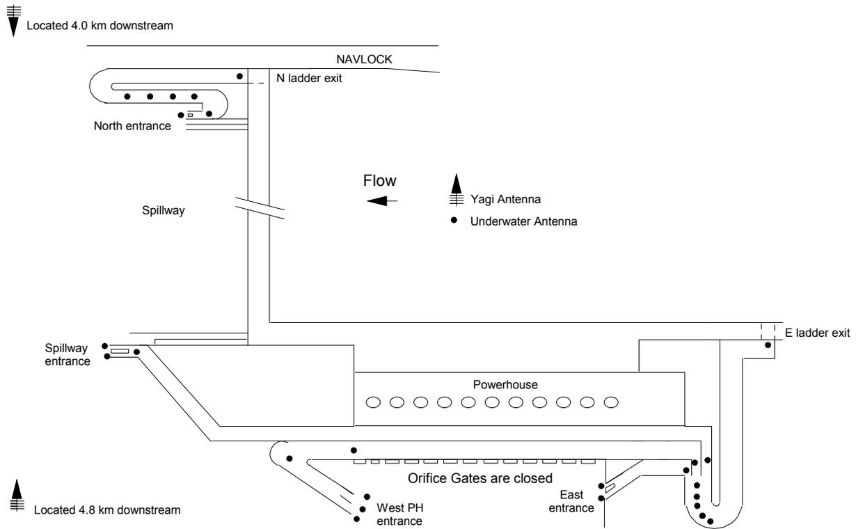
Figure 6. Diagram showing radio antenna deployments at The Dalles Dam in 2014 (not to scale).
