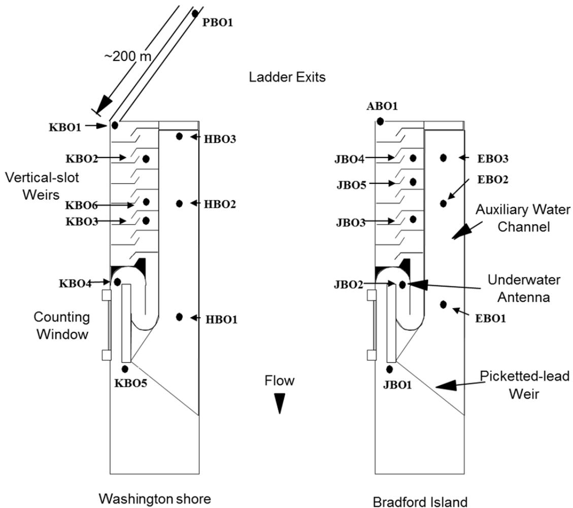
Figure 32. Overhead diagram of radio antenna deployments at Bonneville Dam count stations, serpentine weirs, and auxiliary water supply (AWS) channels in 2014.
