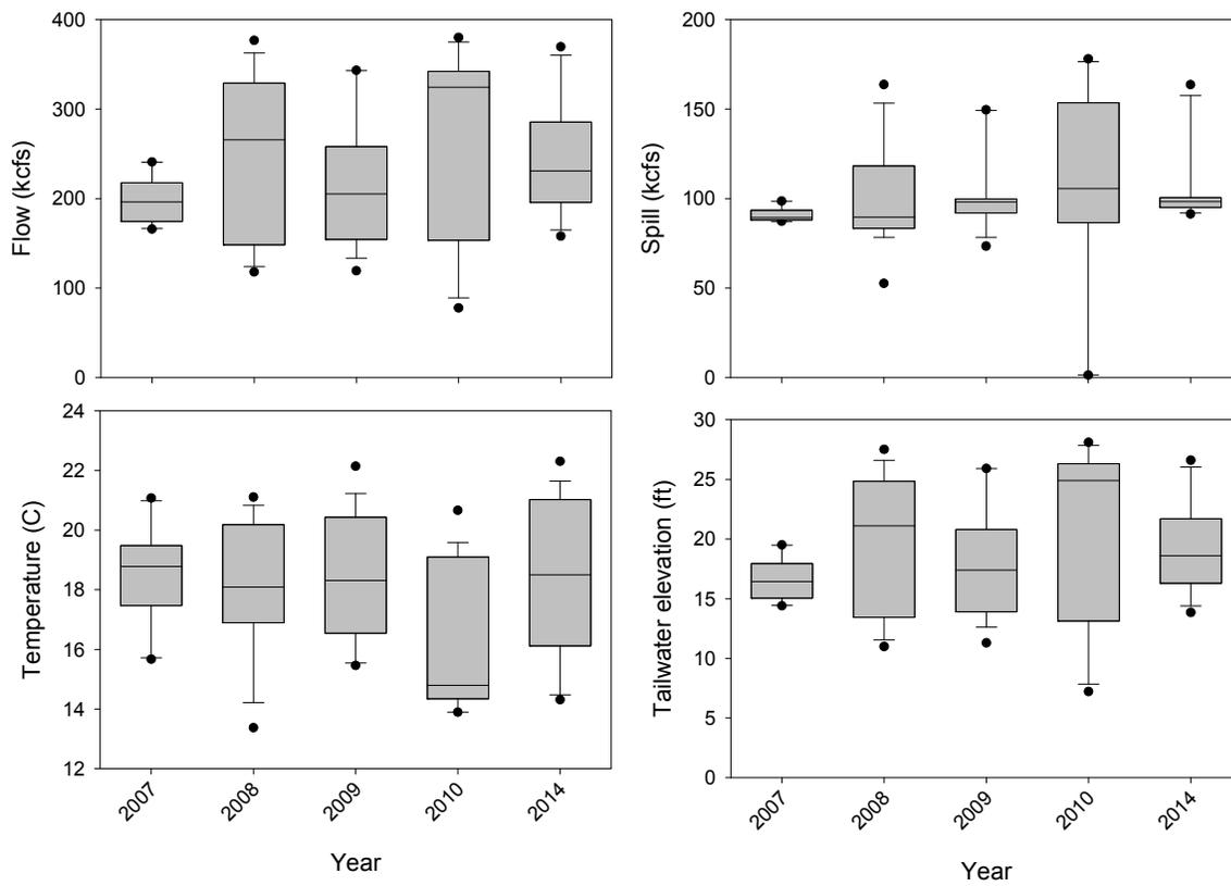
Figure 21. Box plots of the total discharge ('flow'), spill, water temperature, and tailwater elevation on the days that radio-tagged adult lamprey first approached the NDE. Distributions show 5<sup>th</sup>, 10<sup>th</sup>, 25<sup>th</sup>, 50<sup>th</sup>, 75<sup>th</sup>, 90<sup>th</sup>, and 95<sup>th</sup> percentiles.
