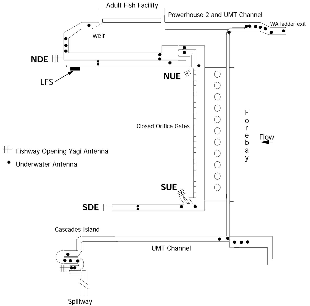
Figure 5. Diagram showing radio antenna deployments at Bonneville Dam PH 2 and Cascades Island in 2014 (not to scale). See Figure 9 for LFS details.
