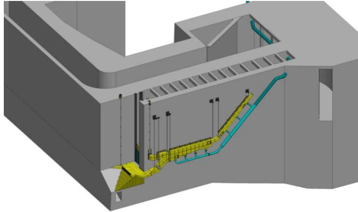
Figure 1. Lamprey flume system (LFS) designed for the Washington-shore NDE.
