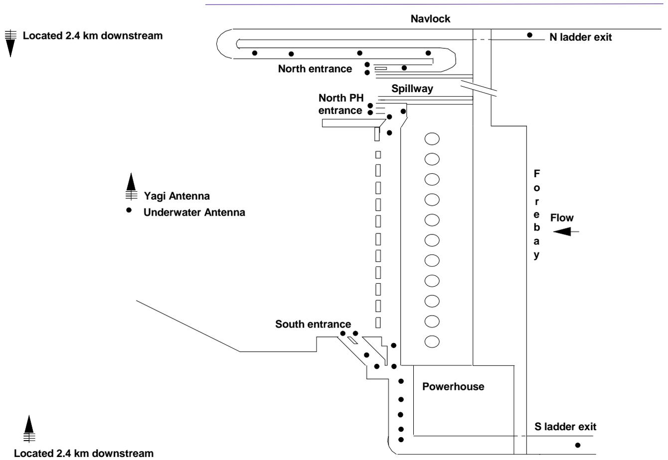
Figure 8. Diagram showing radio antenna deployments at McNary Dam in 2014 (not to scale).
