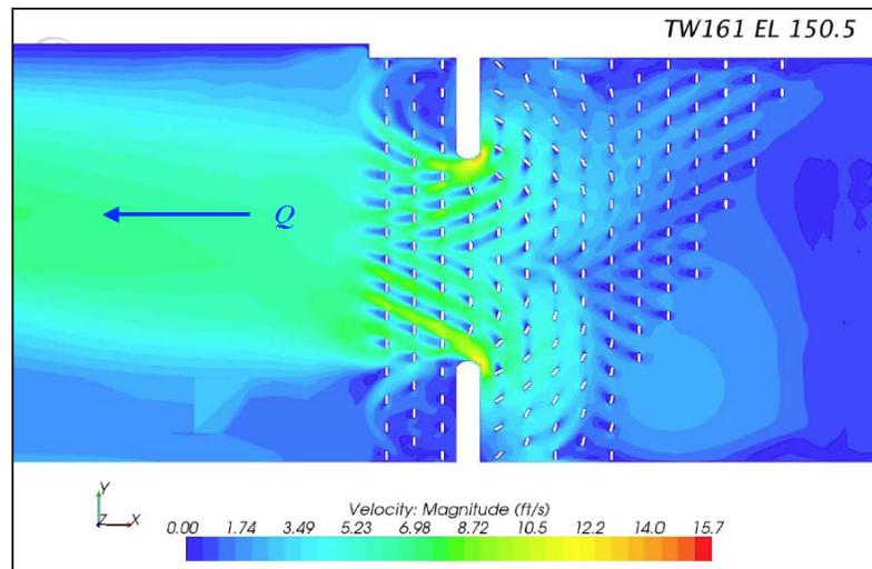
Figure 36. Velocity contours on horizontal plane (6" above invert) with elongated, rotated bollard configuration at the John Day north entrance. Q = flow direction (Source: Yin et al. 2010).
