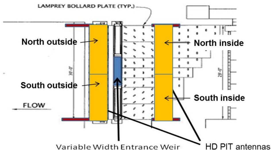
Figure 35. Overhead diagram of HD-PIT antenna array at the John Day north entrance in 2014.
