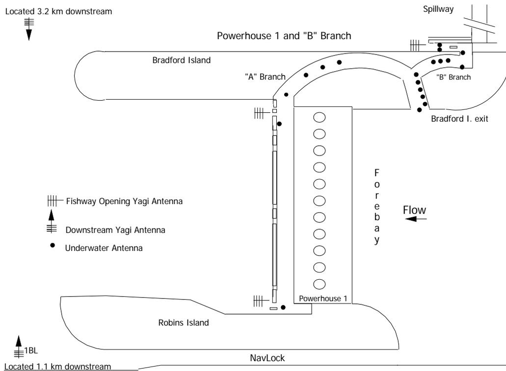
Figure 4. Diagram showing radio antenna deployments at Bonneville Dam PH1 and B-Branch fishways in 2014 (not to scale).
