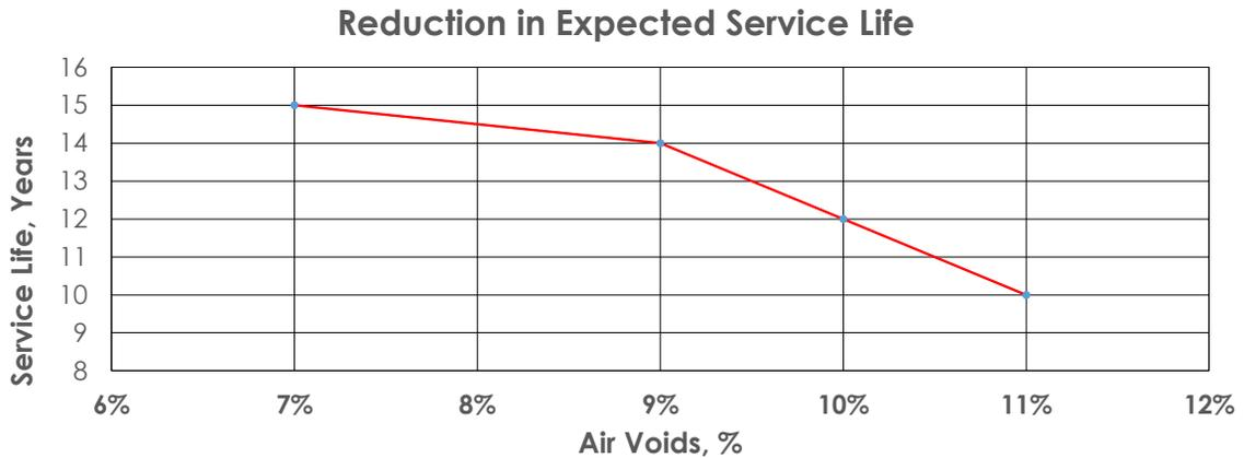
If the center of the mat is at 7% voids or less, but the joint is at 11% voids, the joint fails 5 years earlier than the rest of the pavement.
