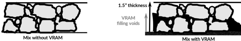
Cross Sectional View at Longitudinal Joint
