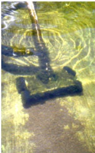
**Picture 2. Vacuum head mounted on wheels; notice the settled material in the foreground.**
