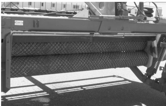
**Figure 9.4.** A super conditioner uses air pressure cells to provide about 2,300 pounds of force on each side of the rolls, and a hard flat plastic surface to flatten the entire stem.
