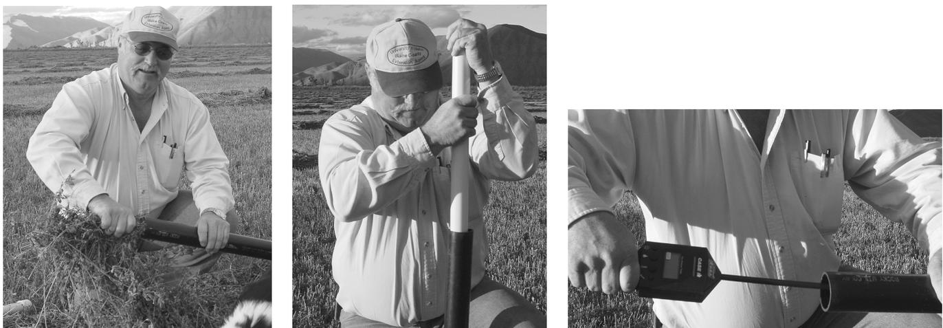
**Figure 8.3.** Steps in using the windrow sampling tool. From left to right: twisting folded hay into the tool, compressing the hay with a plunger, taking moisture readings at depths of 4, 8, 12, and 16 inches in the cylinder.
