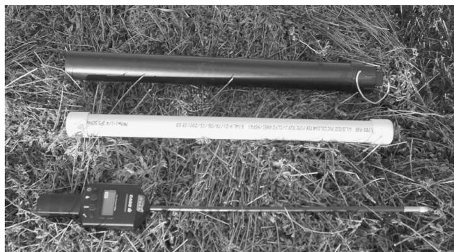
**Figure 8.2.** The windrow sampling tool developed by Ron Thaemert improves the accuracy of windrow moisture detection.
