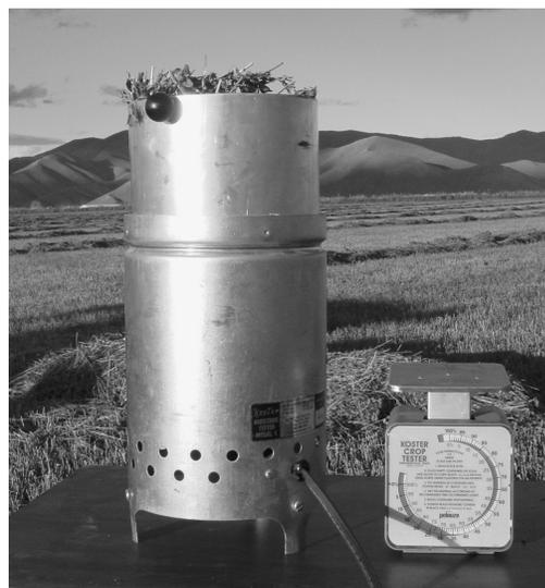
**Figure 8.1.** The Koster field drier can be used to determine forage moisture content.
