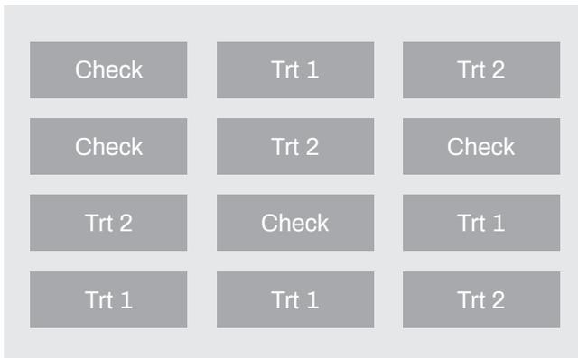
**Figure 2.** Completely Randomized Design plot layout with three treatments (check, trt 1 and trt 2) replicated four times.
